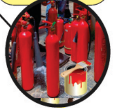
(iii) Deliberately not emptying expired powder before Recharging to get desired reading of the pressure gauge
